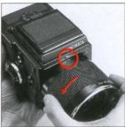
B. The Tele-Converter is attached to the body in the same manner that the lens is attached to the body. (See page 22 of the Instructions for the SQ-Ai.) First, rotate the film winding crank and cock the lens shutter. Next, align the orange dot on the body with the red dot on the Tele-Converter and insert the latter. Rotate in a counter-clockwise direction until it stops with an audible click.
