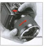
C. To detach the Tele-Converter from the body, press the lens release button (on the left side of the body) down and, at the same time, rotate the Tele-Converter in a clockwise direction until it makes a full stop and can be detached.
