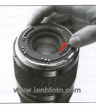
C. Since the cocking pins of the Tele-Converter will return slightly towards the release position (de-cocking slightly) upon detachment from the body, move the cocking pins to the green dots manually.
