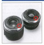
A. First, check whether the cocking pins on the rear surfaces of the Tele-Converter and prime lens are all positioned between the green dots and red bands. If not, move the cocking pins manually to the green dots.
