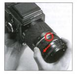
C. In the same manner, first, check whether the cocking pins are positioned between the green dots and red bands, when attaching prime lens to the Tele-Converter. Then, align the red dot on lens to the orange dot on the Tele-Converter and insert lens in fully. Rotate lens in a counter-clockwise direction until it stops with an audible click and is securely attached.
